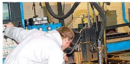
Fig. 3 — Student Phillip Henney, Huntington, Pa., CNC plasma arc cutting.
